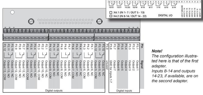
Fig. 4-24: Terminal blocks for digital inputs and outputs
